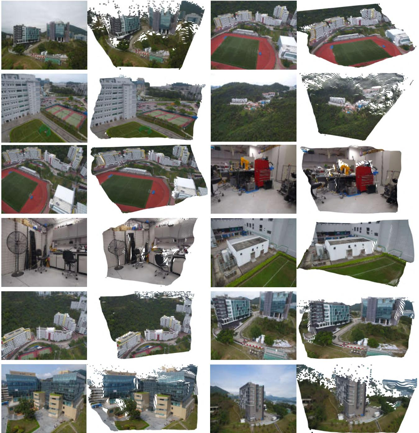
Fig. 6. Corresponding point cloud visualization of the estimated depth maps in Figure 5. In each sample, left is the source image and right is the rendered point cloud. Pixels with depth larger than 200 are considered as the sky and not visualized.
